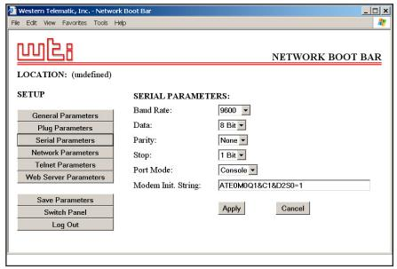
Figure 5.5: Serial Parameters Menu - Web Browser Interface
